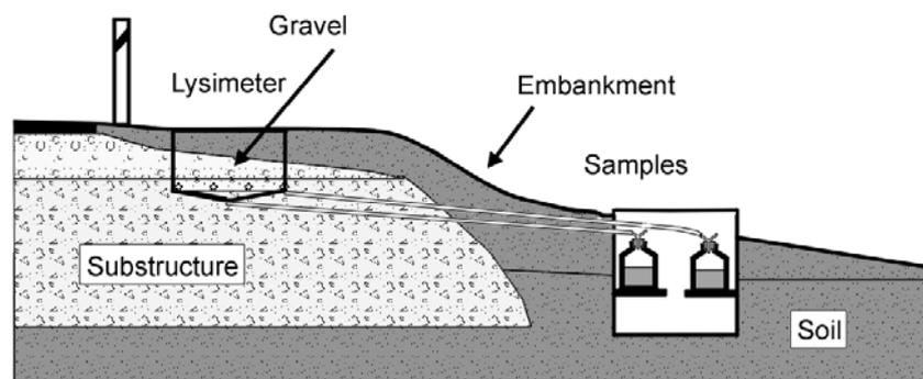
Fig. 2: Schematic crossection of lysimeter installation and sampling
