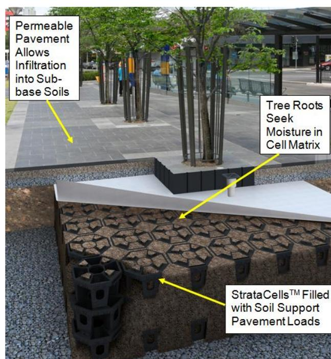
Figure 4. Typical StrataCell<sup>TM</sup> Application (<http://www.citygreensystems.com>)
